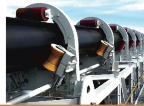
Pipe Conveyor Belts
